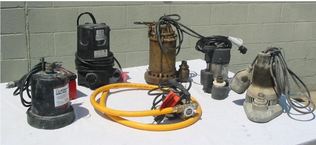
Sump & transfer pumps
