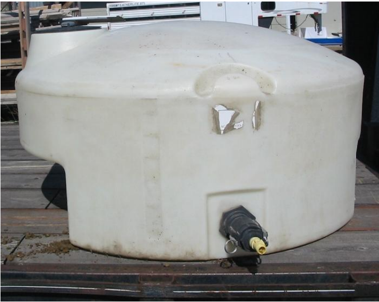
150 Gallon water tank
