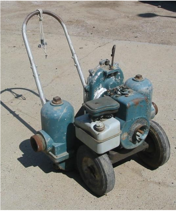
Trash pump with intake & discharge hoses
