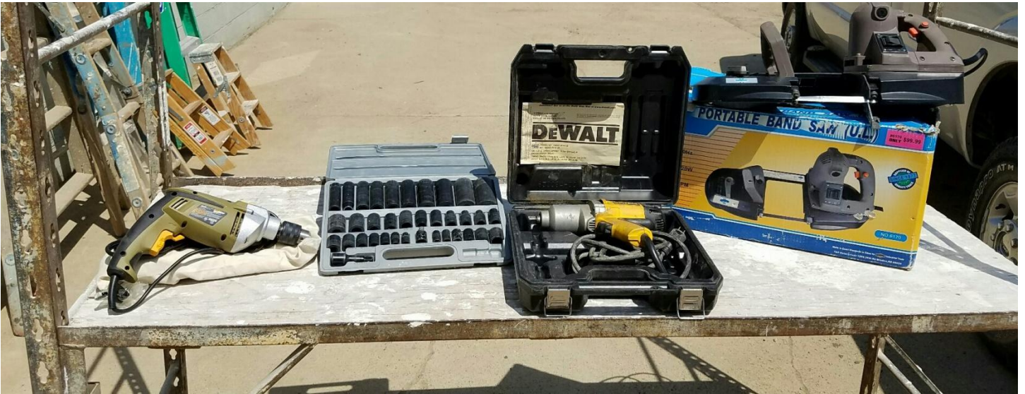
\frac{1}{2} " Electric impact wrench, \frac{1}{2} " & \frac{3}{8} " Impact sockets, \frac{1}{2} " hammer drill, Portable Band Saw
